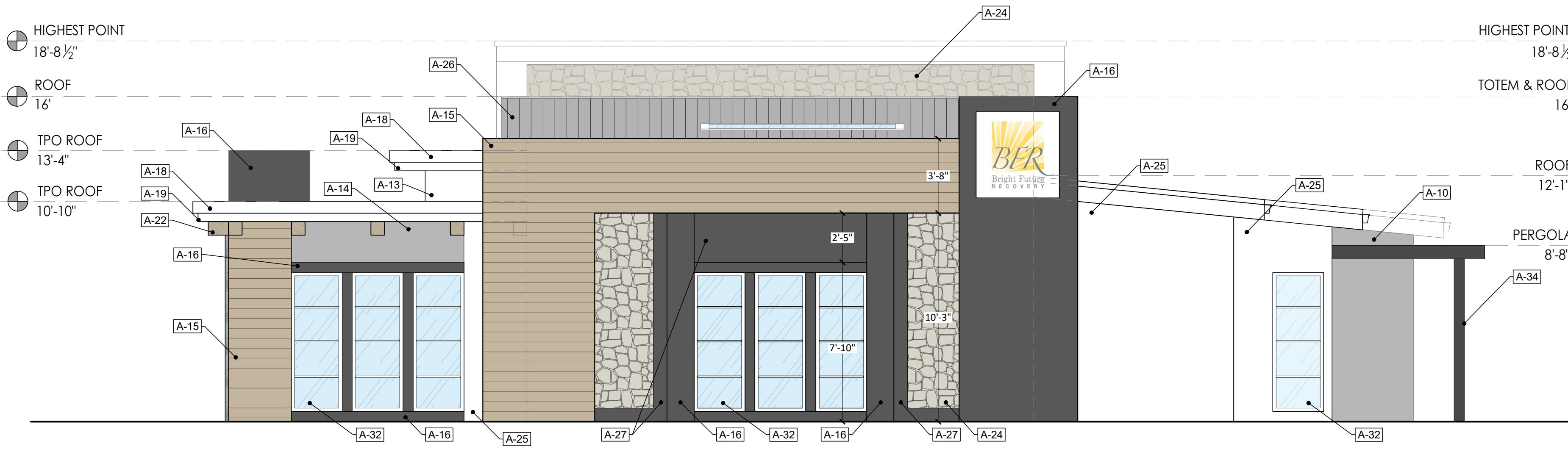
ADMIN-BUILDING MAIN HOUSE - FRONT ELEVATION
