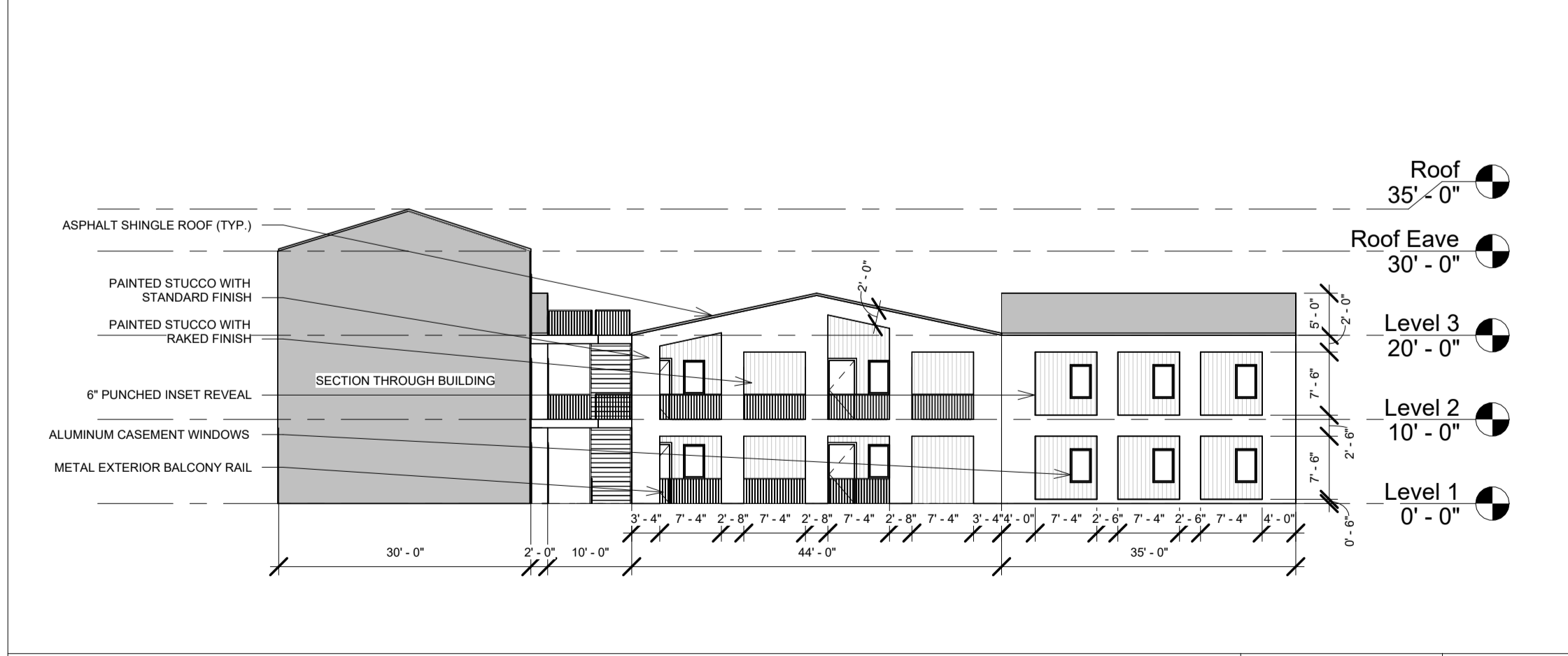
Building C Courtyard South Elevation 1/16" = 1'-0" 3 A-202
