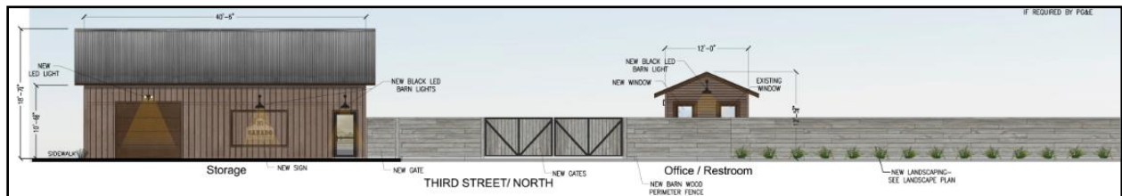
Figure 4 – North Elevations Cont.
