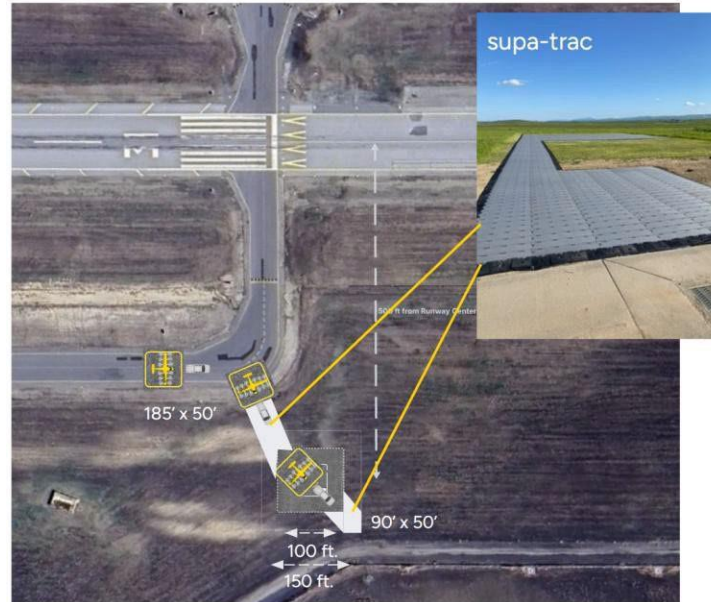
Figure 2-3: Temporary Surface Area for Towing
